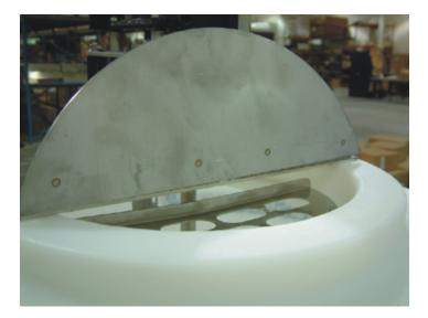
**Step 4:** Ensure the tank valves are in the RINSE mode. Gravity will drain the tank. Repeat filling and draining the Tank until thoroughly clean and empty.
