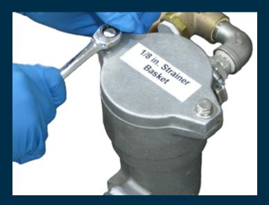
**Step 3:** Remove the filter screen from the filter bottom and check it for clogging and material build-up. Clean it thoroughly.
