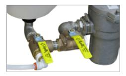
**Step 8:** Remove the hose with 3/4" Male fitting from the Drain Valve.
