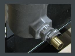
Step 2: Connect the other end of the Tubing to the BT Pump Brass Hose Barb on a Pump & Weighing Station with Hose Clamp. Tighten in place with a screwdriver.
