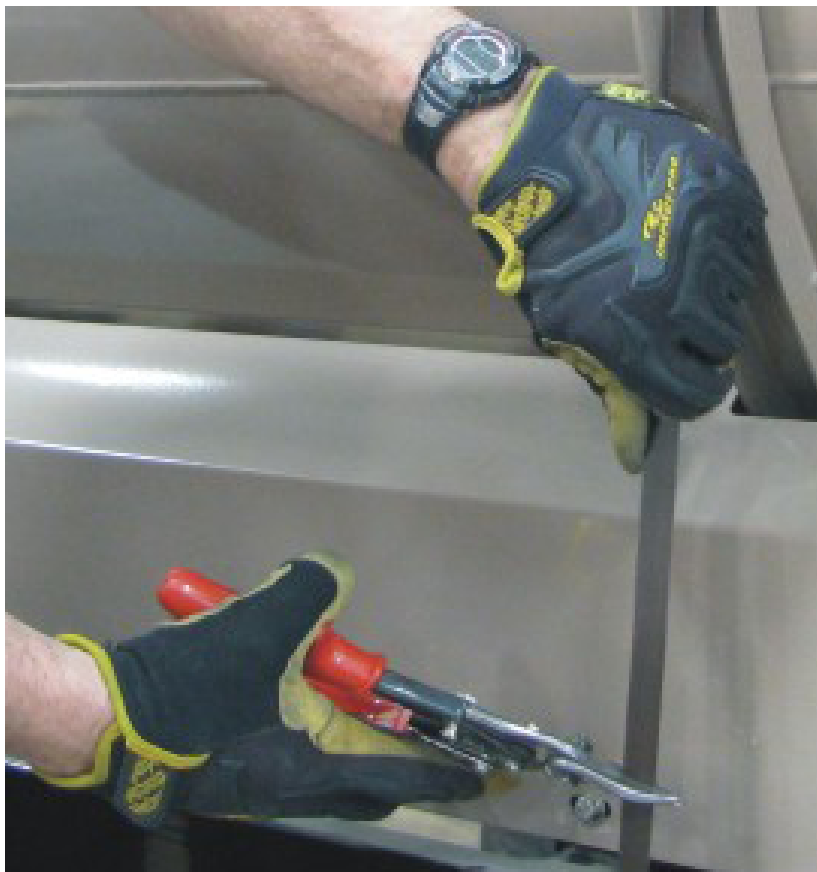
Use safe hand placement to cut the Drum bands, ref.
